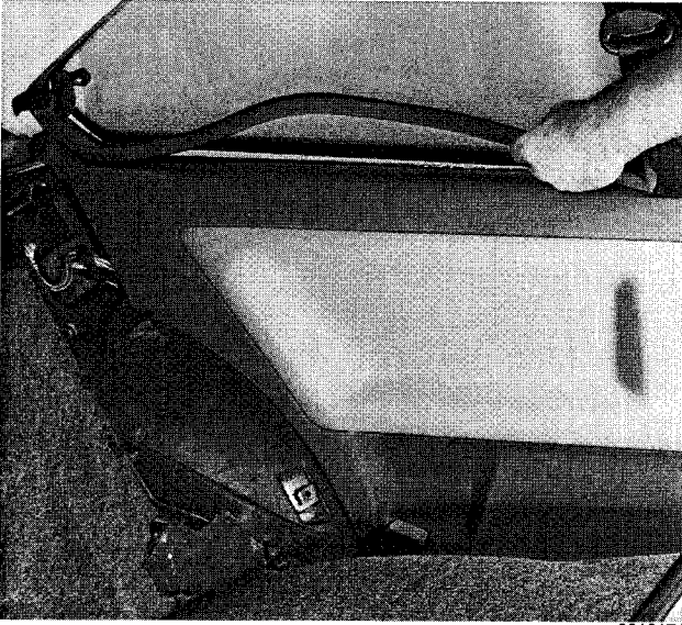
Fig. 10. Panel edge trim piece trim being removed.
