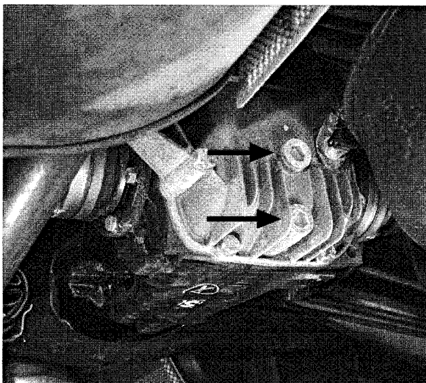
Fig. 26. Final drive oil filler and oil drain plugs.
