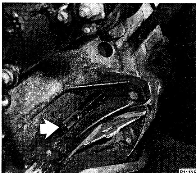
Fig. 11. BMW special tool no. 11 2 300 installed through bellhousing and into flywheel (arrow) to lock crankshaft at TDC.
