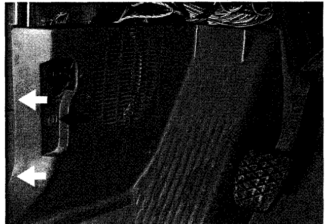
Fig. 7. Rotate plastic retainer ( black arrow ) and remove panel in direction shown ( white arrows ).
