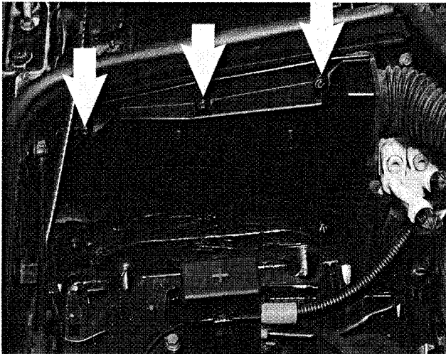
Fig. 16. Engine control unit (ECM) compartment cover screws (arrows).
