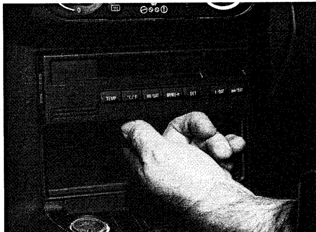
Fig. 9. Removing the Multi-Information Display (MID) module.
