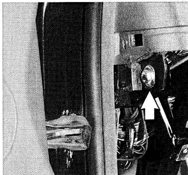
Fig. 10. Dashboard mounting bolt (arrows). Left side shown, right is similar. Some models may have two bolts on each side.
