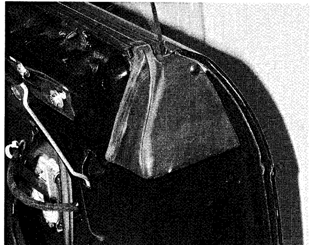
Fig. 15. Correct installation of door top rubber seal.
