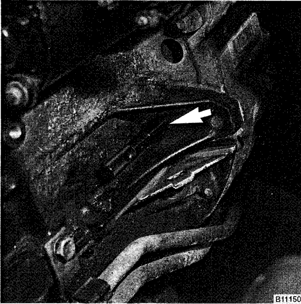
Fig. 36. BMW special tool no. 11 2 300 installed through bellhousing and into flywheel.
