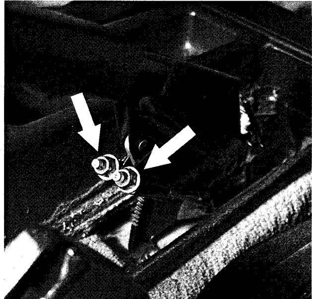
Fig. 15. Parking brake cable adjusting nuts (arrows).
