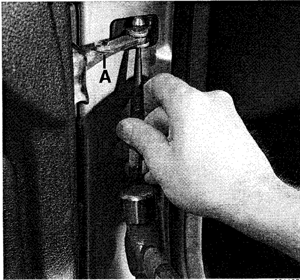
Fig. 3. Door check pin being removed. Note retainer clip (A) used on early models.
